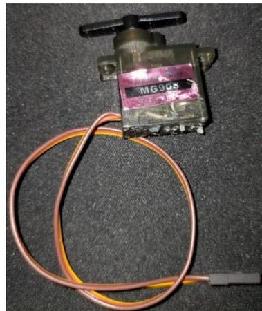
**Gambar :** Motor Servo MG90S
