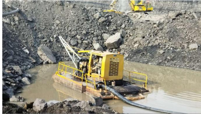
**Gambar 4.7 Pompa Mf-290**
