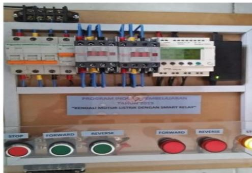
**Gambar 4. Uji Coba Kontrol Forward Reverse**
